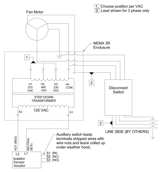
This diagram is NOT to be used with a VFD.
