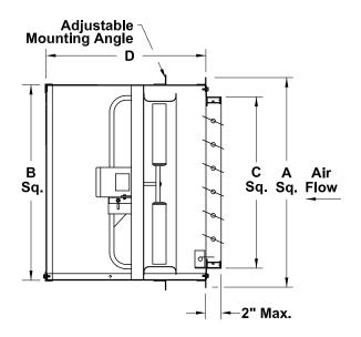
Note: Correct propeller rotation is CCW when viewing from inlet side.
